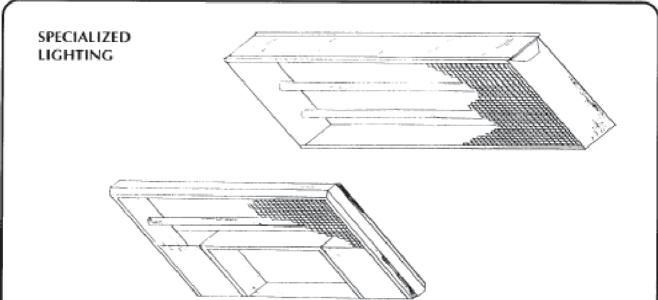
Canopy Lighting available with either solid or open frontal panel for transparent backlit signage. All canopies custom made to specifications.
